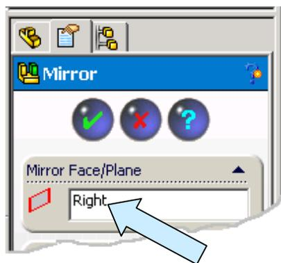
Notice that the right plane is automatically entered in the Mirror Face/Plane Field in the left pane.
